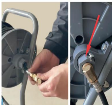
Connect the main hose to the short one and secure them with a short screw. remain outside.
